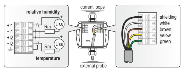
The loop resistance value Rc = Rm + resistance of wires must fulfill the condition  $Rc[\Omega] < 40 \times Uss[V] - 360$ .
