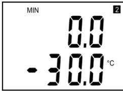
Range and type of value for output 1 (Uout 1 = symbol „1“ on display). Type of value, assigned to output 1, is indicated by displayed unit (here °C). Upper line displays voltage value corresponding to measured value (lower line). Here 0V corresponds to ambient temperature -30 °C.
