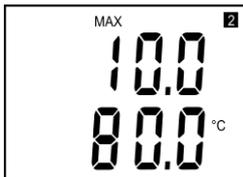
After next press of the button value for upper point appears, here 10 V corresponds to ambient temperature +80 °C.
