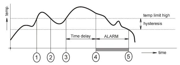
An alarm report is always sent right after an alarm appears. The device memorizes sent alarm reports of current alarms while the power is connected. In case of power disconnection or a reset of the device (e.g. by modification of configuration) a new alarm evaluation is performed and new alarm reports are sent again, if any.
