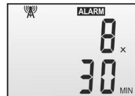
**8x** - shows how many times the regular message will be sent before the new transmitter setup (if this requirement is currently set in the cloud). The information is reduced with each regular report sent. Reading the new settings from the cloud occurs when the display shows "1x 0 min". If the remote setting is in the device disabled, this line is not displayed.
