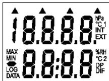
Switch ON the instrument by pressing ON/OFF key. After switching ON the instrument all symbols on the LCD are displayed. If the ON/OFF key is being held pressed, all LCD symbols are displayed till the key is released. In usual operation instrument then starts the measurement mode and actual measured values are displayed.
