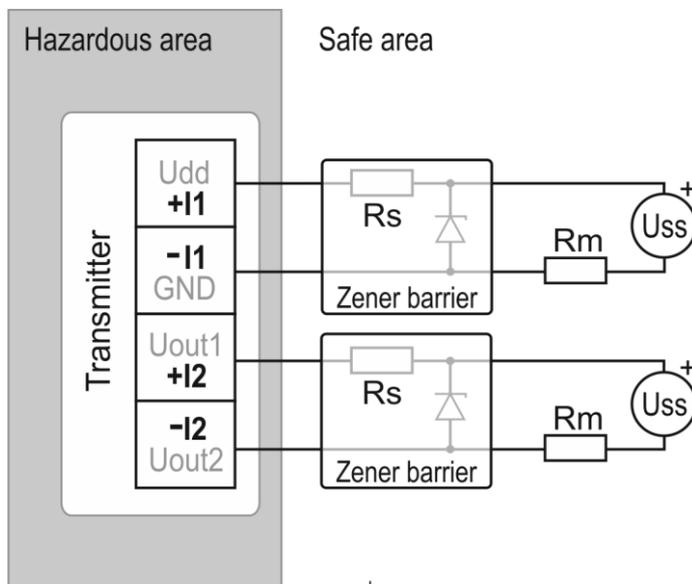
Loop resistance value  $R_c = R_m + R_s + \text{resistance of wires}$  shall fulfill the condition  $R_c[\Omega] < 40 \times U_s[V] - 360$ .
