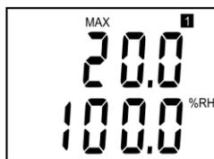
Press button again to get value for upper point of the 1. output (here „%RH“ = relative humidity and „1“ = loop I1). Upper line displays value of the current corresponding to measured value on the lower line (here 20 mA corresponds to 100 %RH).
