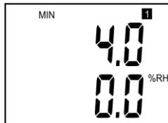
The LCD display shows the type of value assigned to 1. output (here „%RH“ = relative humidity and „1“ = loop I1). Upper line displays value of the current corresponding to measured value on the lower line (here 4 mA corresponds to 0 %RH).
