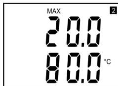
Press button again to get value for upper point of the 2. output (here „°C“ = temperature and „2“ = loop I2). Upper line displays value of the current corresponding to measured value on the lower line (here 20 mA corresponds to 80 °C).
