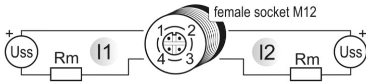
Loop resistance value  $R_c = R_m + \text{resistance of wires}$  shall fulfill the condition  $R_c[\Omega] < 40 \times U_{ss}[V] - 360$ .
