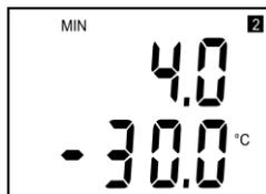
After next press of the button LCD display shows the type of value assigned to 2. output (here „°C“ = temperature and „2“ = loop I2). Upper line displays value of the current corresponding to measured value on the lower line (here 4 mA corresponds to -30 °C).
