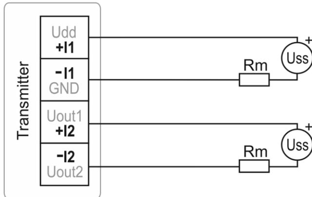
Loop resistance value  $R_c = R_m + \text{resistance of wires}$  shall fulfill the condition  $R_c[\Omega] < 40 \times U_{ss}[V] - 360$ .
